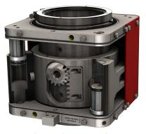
Inner rotating and outer stationary assemblies separate the hydraulics from the drill string **eliminating the need for rotary hydraulic seals**. As the hydraulics are isolated from the drill string, the actuator can be functioned while the drill stem is rotating
